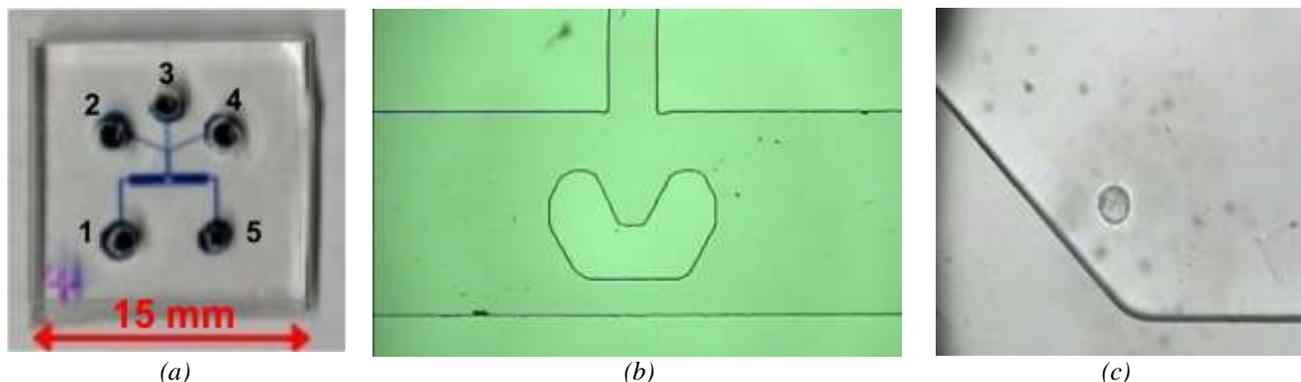
Fig. 1. The microfluidic biochip. (a) Image of the microchip with channels filled with a blue food dye for easy visualization. PDMS chip showing reservoirs 2, 3, 4 used for drug delivery, reservoir 1 as the cell inlet and reservoir 5 as the waste, (b) region of the central chip chamber showing the cell retention structure, (c) The close-up of the chamber with cell retention structure. As shown, a single NCI-H1650 cell retained within the retention structure
